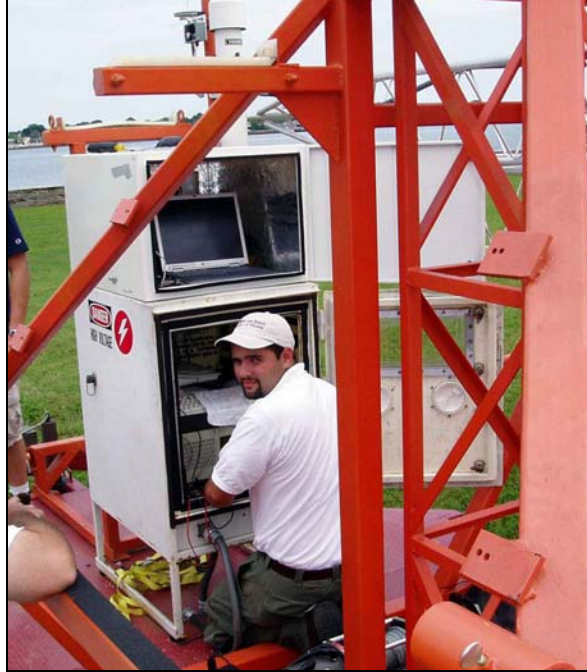
Figure 2-2. Mobile Tower computer box after modification for 2003 hurricane season. Testing at the Castillo de San Marcos (St Augustine, FL) with the cooperation of the National Park Service, an FCMP team from the University of Florida tested the new real-time data acquisition system on July 16, 2003.
