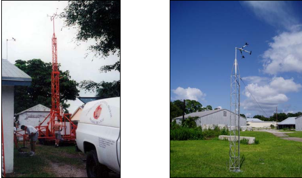
Figure 1-1. Mobile tower FCMP deployment for hurricane Michelle during 2001 hurricane season (left). Satellite tower testing at Florida Department of Transportation in Gainesville, FL (right).
